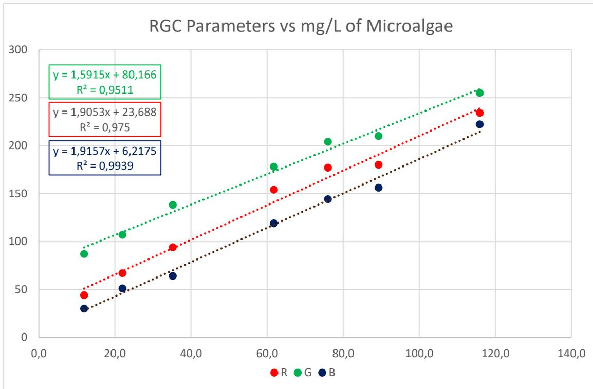
Table 2. Results of dry microalgae mass vs. RGB image decomposition parameters.
