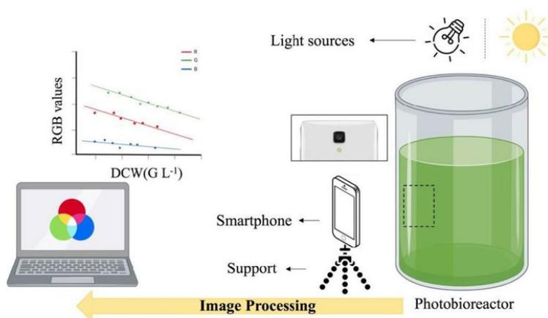
The sizes of the captured images were 4160×3120 pixels. Then, they were uploaded to a laptop to perform color decomposition by a RGB algorithm, using the **Pillow Python** image processing library. The experimental setup is shown in Fig. 1.
